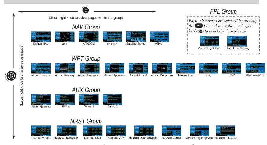
Selection of any main page is performed using the large ( ) and small ( ) right knobs. The large right knob ( ) selects the page group: NAV, WPT, AUX or NRST. The small right knob ( ) selects the desired page within a group. To quickly select the default NAV page, press and hold .
